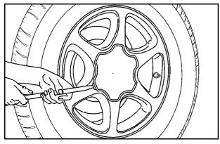
2. If your vehicle has a center cap that covers the wheel fasteners, place the chisel end of the wheel wrench in the slot on the wheel and gently pry the cap out.
